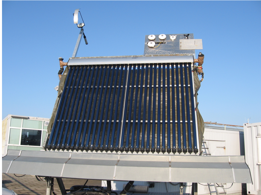
Figure 1: Picture of the collector Solos Modello Mela 30R mounted on the test facility of Fraunhofer ISE
